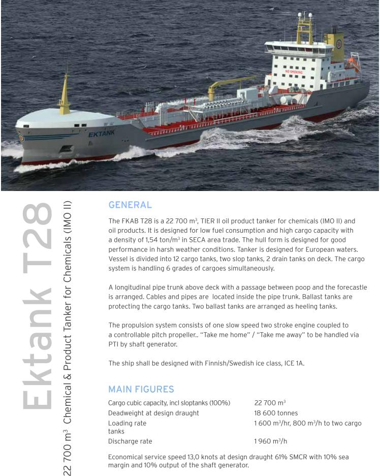
The FKAB T28 is a 22 700 m<sup>3</sup>, TIER II oil product tanker for chemicals (IMO II) and oil products. It is designed for low fuel consumption and high cargo capacity with a density of 1,54 ton/m<sup>3</sup> in SECA area trade. The hull form is designed for good performance in harsh weather conditions. Tanker is designed for European waters. Vessel is divided into 12 cargo tanks, two slop tanks, 2 drain tanks on deck. The cargo system is handling 6 grades of cargoes simultaneously.
