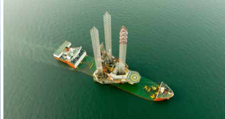
Aframax converted to Semisubmersible Vessel
